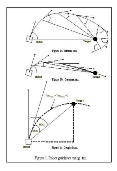
for the robot soccer domain as it enables the robot to place itself behind its target (a ball) in order to manoeuvre it towards a goal.
